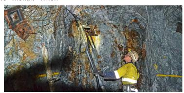
Using an 'airleg' as part of narrow vein mining.
