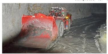
A 'baby bogger' in a  $5m \times 5m$  drive (tunnel).
