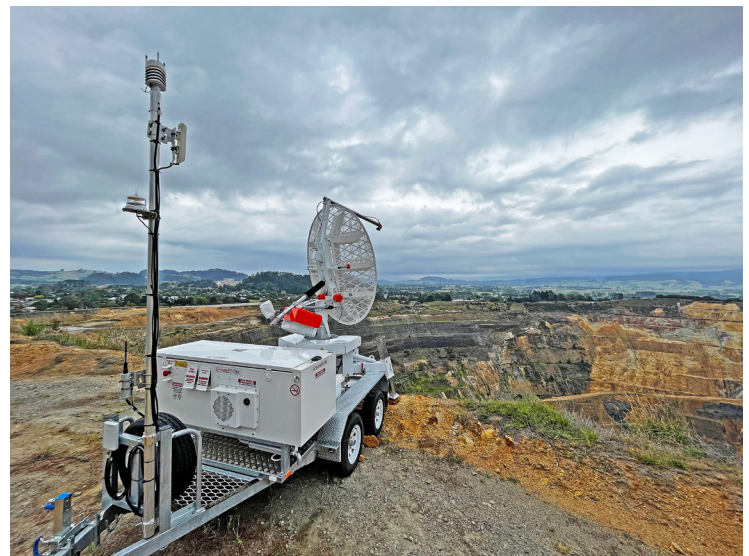
The Radar used to constantly monitor the Martha Open Pit.
